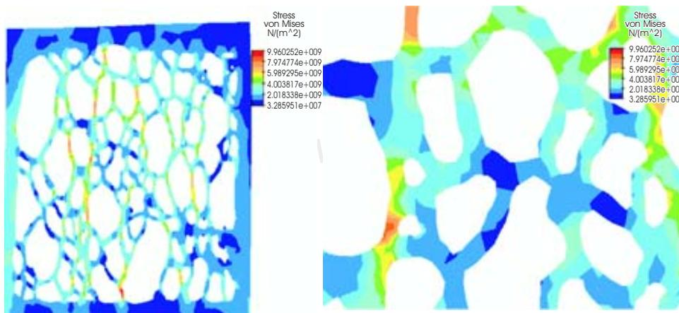
Figure 3. A trabecular section at compression loading.
