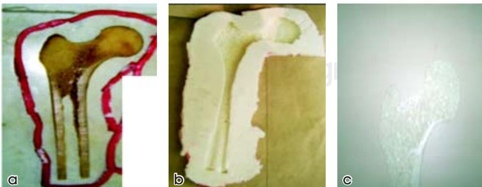
**Figure 1.** Plaster casting molding. a) Histological sample; b) Silicon mold; c) photoelastic model.
