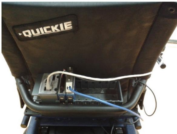
Figure 18. NI Compact-RIO installed for the real-time system.
